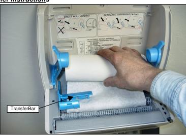
2) Carefully remove the stub roll, making sure the paper web is under the transfer bar.
